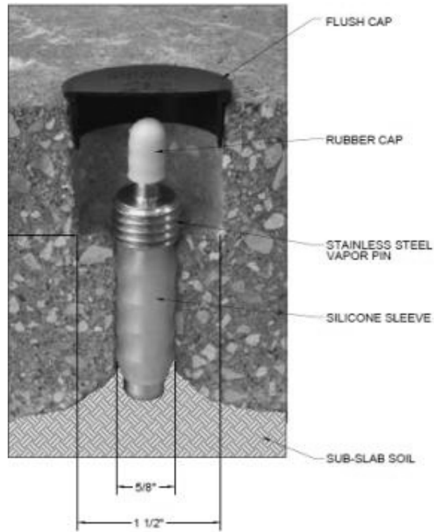
Permanent, flush-mounted sample points installed through slab
