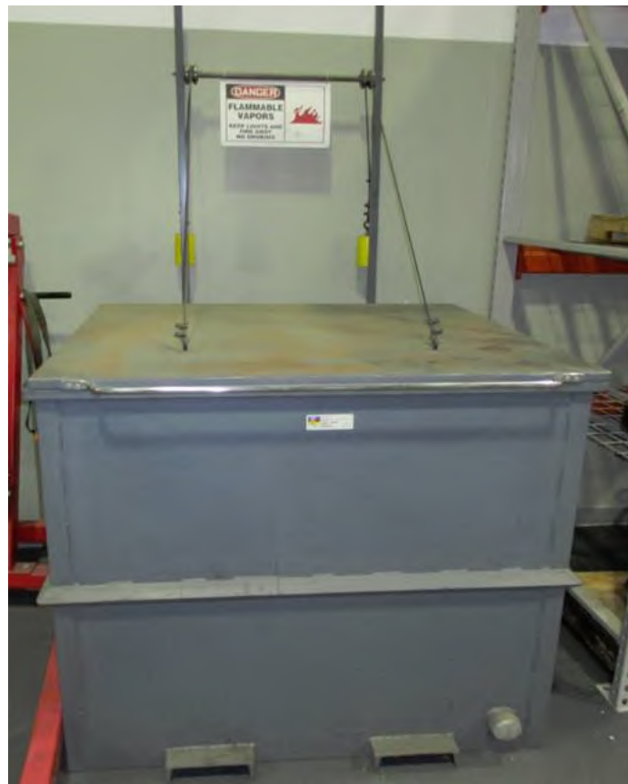
Figure 8. Aerosol recycler/can crusher.
