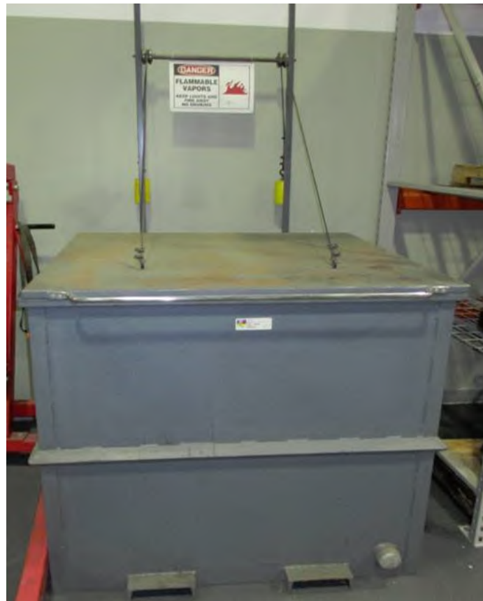
Figure 8. Aerosol recycler/can crusher.
