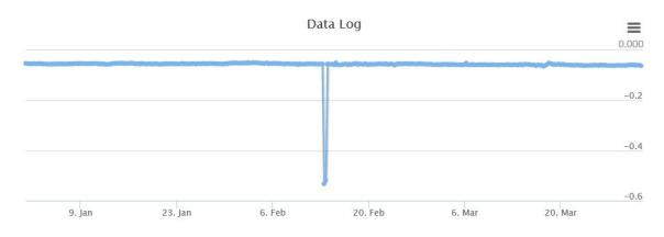
On February 13, 2023 there was a neighborhood wide power outage due to a storm event which resulted in the negative spike seen on the plot above. Below is a zoomed in portion of the data plot starting on February 14, 2023 showing the IPM system continuing to maintain vacuum level at the monitoring point which is typical of normal operation at this property.
