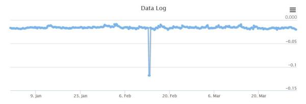
On February 13, 2023 there was a neighborhood wide power outage due to a storm event which resulted in the negative spike seen on the plot above. Below is a zoomed in portion of the data plot starting on February 14, 2023 showing the IPM system continuing to maintain vacuum level at the monitoring point which is typical of normal operation at this property.
