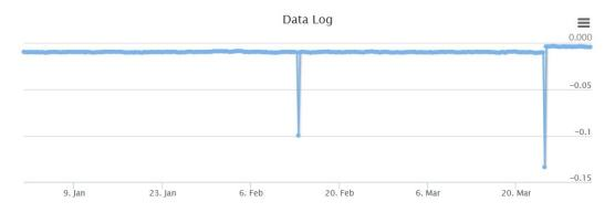
On February 13, 2023 there was a neighborhood wide power outage due to a storm event which resulted in the negative spike seen on the plot above. Below is a zoomed in portion of the data plot starting on March 24, 2023 after recalibration of the vacuum transmitter showing the IPM system continuing to maintain vacuum level at the monitoring point which is typical of normal operation at this property.
