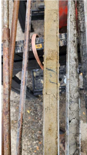
INJ-35-15 ZVI at 9 feet bgs
